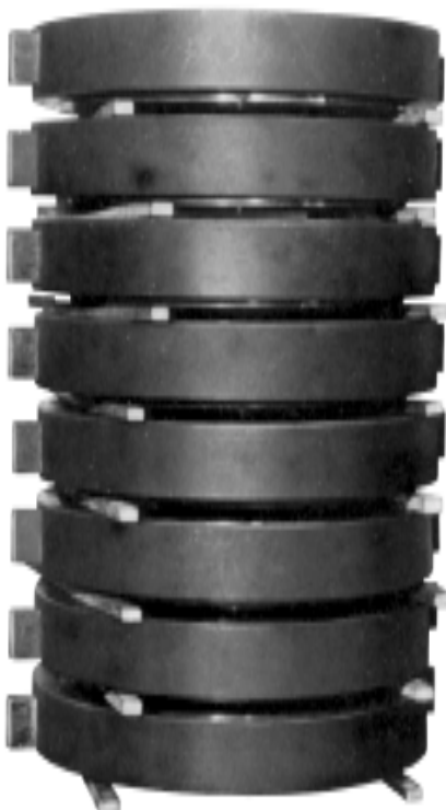
Fig. 43 Stacking the stage casings on top of one another.
