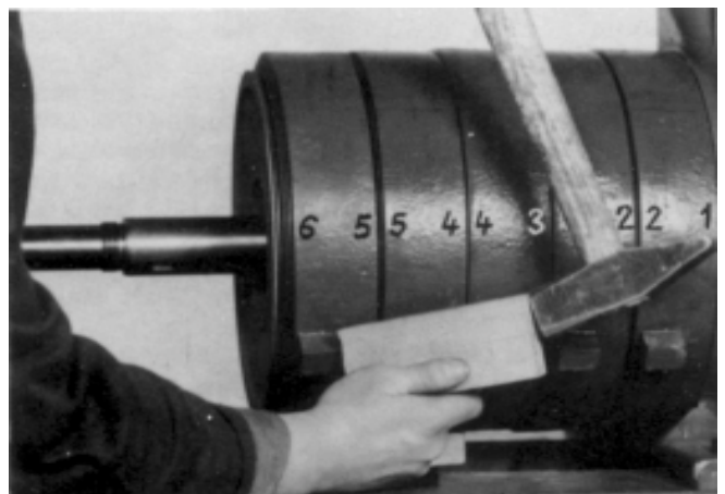
Fig. 40 Slackening and removing the stage casing.
